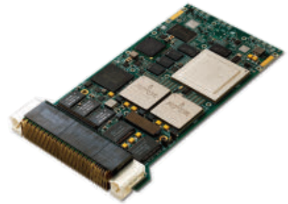
The X-ES XChange3018 is a 3U VPX, 10 Gigabit Ethernet switch module with four 10GBASE-T or XAUI ports, six backplane 10/100/1000BASE-T Ethernet ports, and six backplane network 1000BASE-X Ethernet ports.
